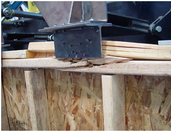
Figure 5: With rods centered in the wall and sheathing on opposite side of wall, cross-grain tension failure occurs as top plate bends upward. Mechanical reinforcement is needed.
