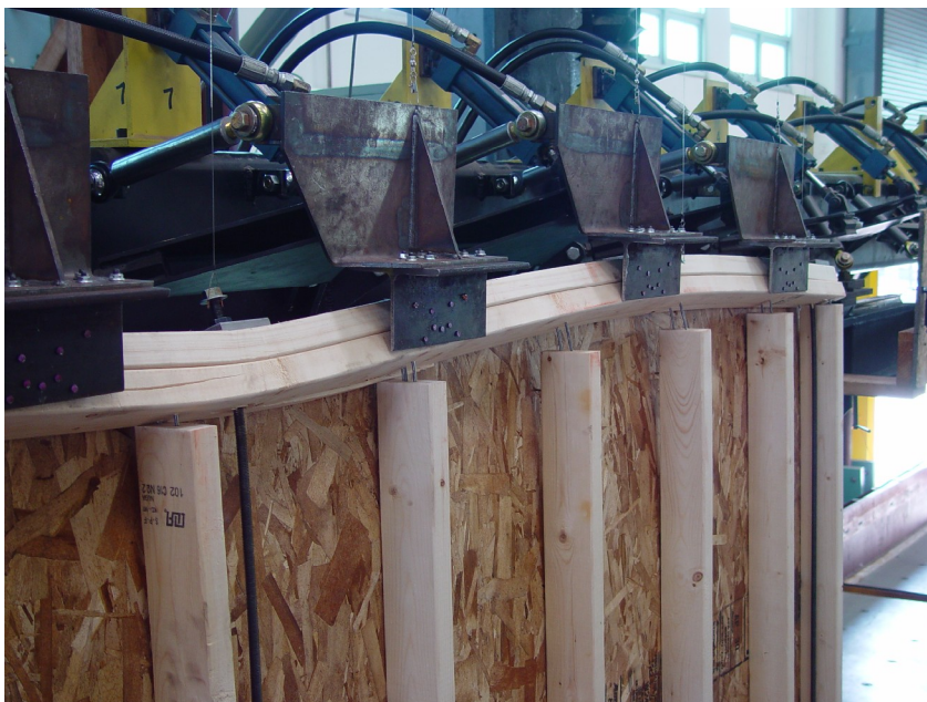
Figure 4: Sheathing and hurricane ties on opposing sides of the wall with rods at 48 inches o.c. Top plate rotation is still unrestrained.
